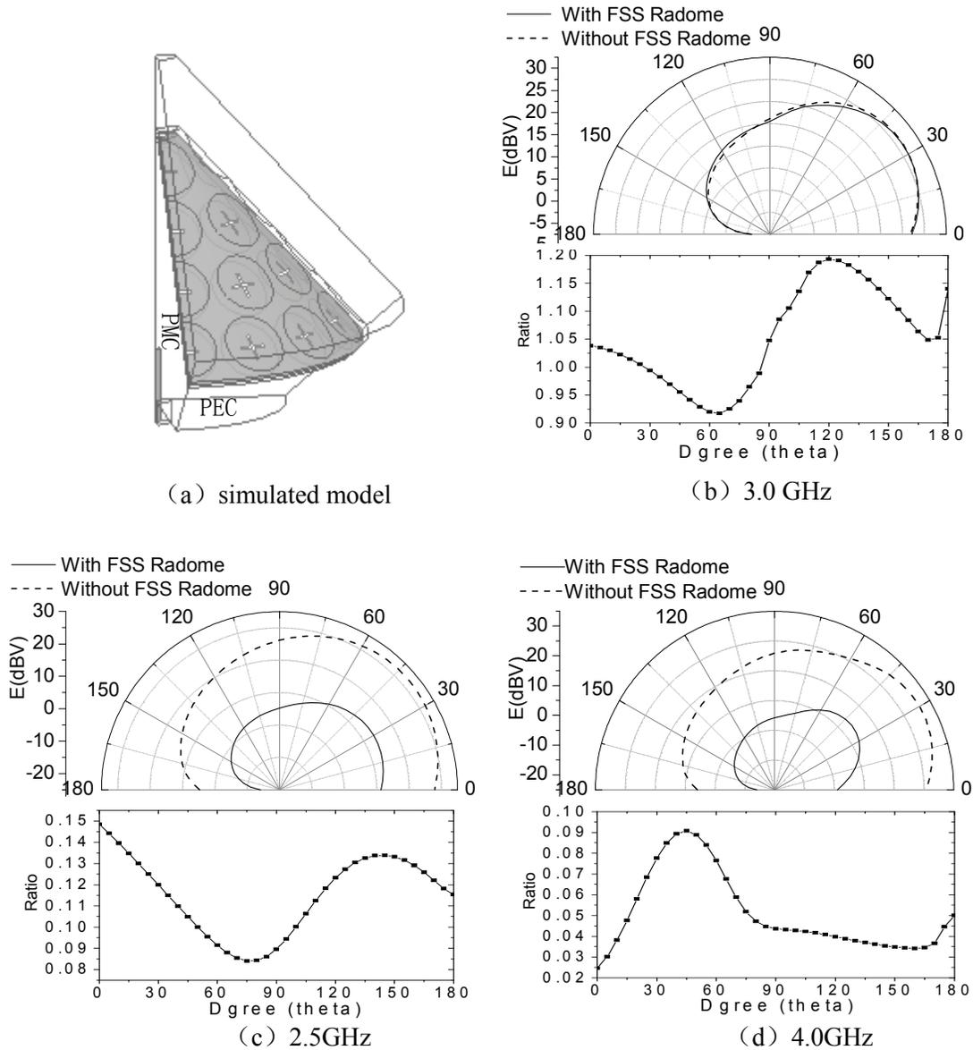
Fig. 4. Three dimensional simulated model of the FSS radome B with a monopole antenna (a) and the simulated results at the three frequencies 3.0GHz (b), 2.5GHz (c) and 4.0GHz (d).
