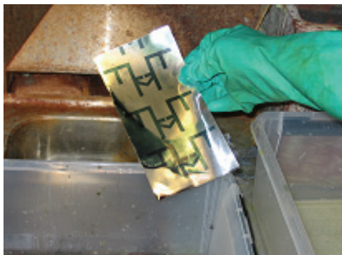
Fig. 3. Placement of varnished aluminum substrate within the solution.
