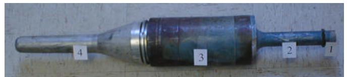
Fig. 1. 120 mm HEAT round UXO consists of four sections, altogether about 80 cm long: 1) magnetic (steel), 2) non-magnetic titanium, 3) steel, and 4) aluminum.
