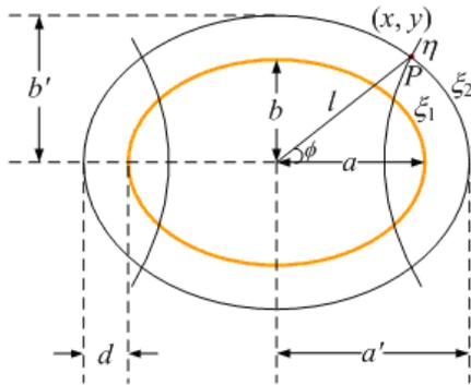
Fig. 1. Cross-section view of the elliptical microring.
