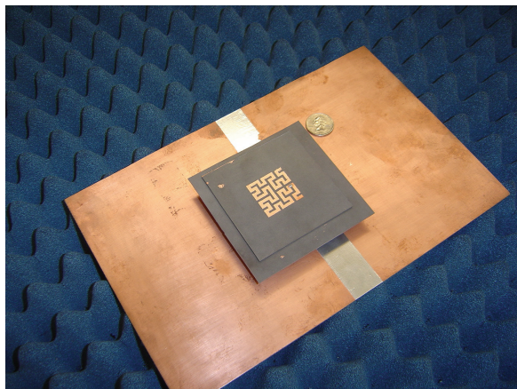
Fig. 22. Prototype of the probe-fed Hilbert antenna above a 4-element Hilbert high-impedance ground-plane.
