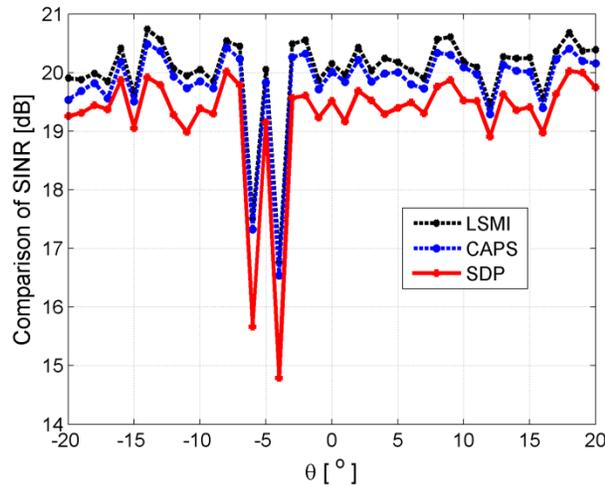
Fig. 7. SINR of three methods, interference at  $-5^\circ$ .
