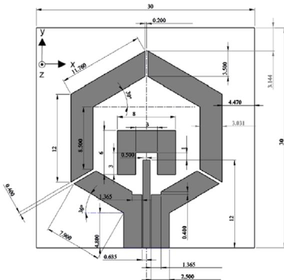
Fig. 1. Geometry of the proposed antenna (unit: mm).
