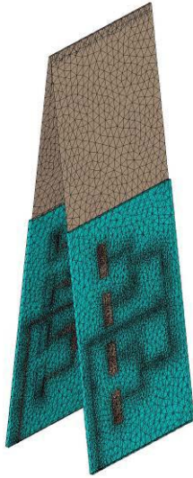
Figure 10. Two 4-element array antennas mounted on a wedge.
