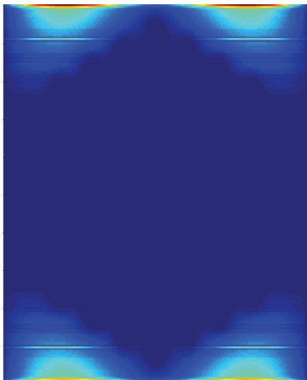
Fig. 5. Magnitude of electrical field of one of the undesired modes: Wave guiding within the PML.
