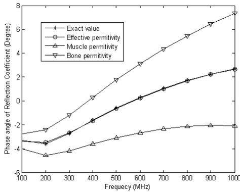
Fig. 3. Comparison of the phase angles of reflection coefficients.
