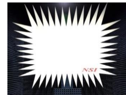
Fig. 6. Realised CATR main reflector.
