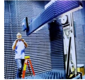
Fig. 11. CATR QZ field being probed using a linear translation stage and a plane-polar acquisition scheme.
