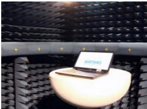
Fig. 2. Microwave Vision Group System to measure small antennas on terminals (MVG copyright).
