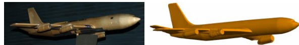
Fig. 1. Boeing 707 scale model in the compact range and laser scanned 3D CAD model in FEKO.
