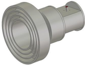
Fig. 1. Model of WR430 CATR feed.
