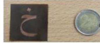
Fig. 5. Photograph of the chipless tag based on the connected Arab letter "خ".
