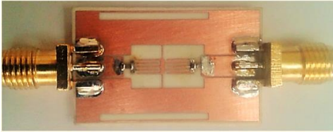
Fig. 8. The fabricated prototype photo of the CPW CRLH filter.
