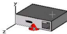
Fig. 10 – Electric field probe's distribution. Three probes are used each one of them for each component of the electric field.
