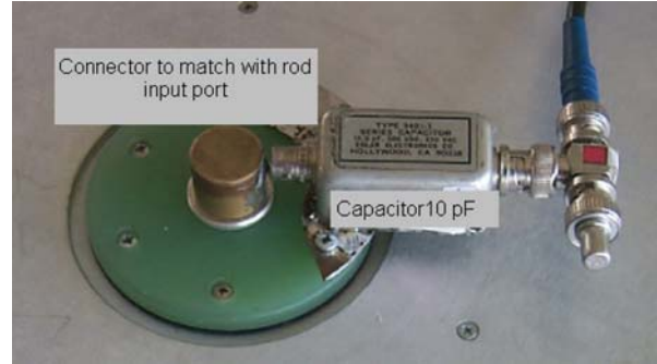
Fig. 2. Test setup of ECISM calibration method.
