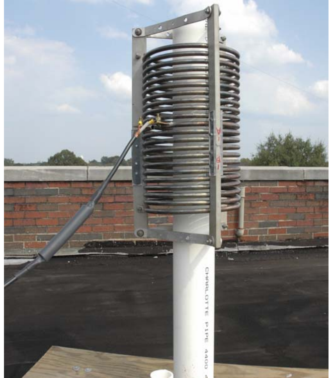
Figure 1. A compact coil (multi-turn loop) antenna.
