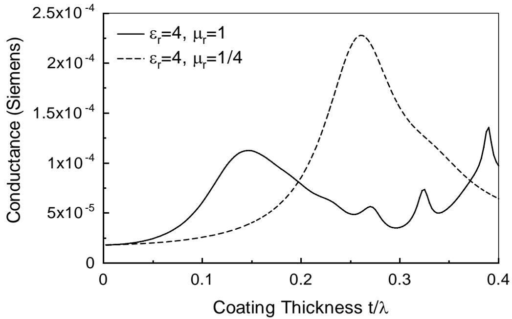
Figure 5: Aperture conductance versus coating thickness for an axially slotted elliptic cylinder coated with conventional and isorefractive materials.
