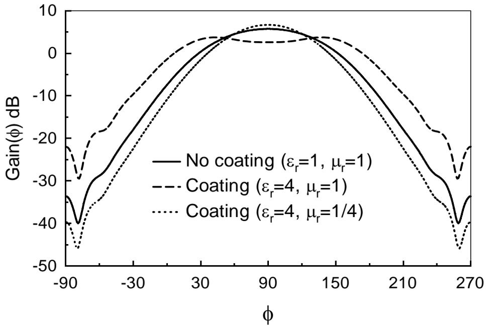
Figure 2: Radiation pattern for an axially slotted elliptic cylinder coated with different types of dielectric materials and coating thickness  $t = 0.15\lambda$ .
