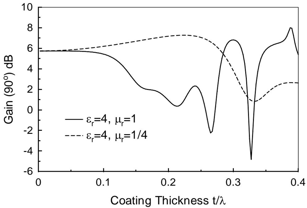
Figure 4: Gain versus coating thickness for an axially slotted elliptic cylinder coated with conventional and isorefractive dielectric materials.
