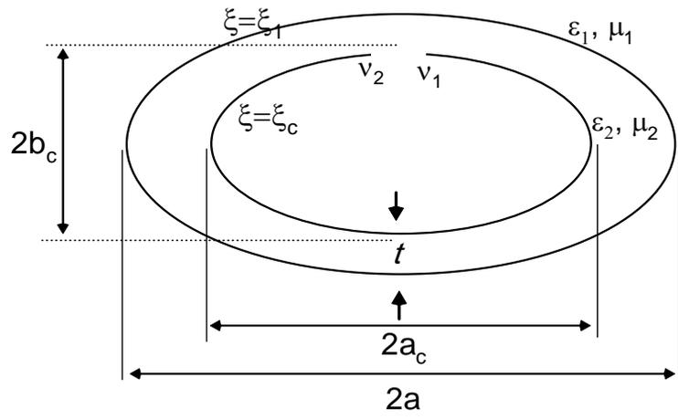
Figure 1: Geometry of axially Slotted antenna on elliptic cylinder with isorefractive layer
