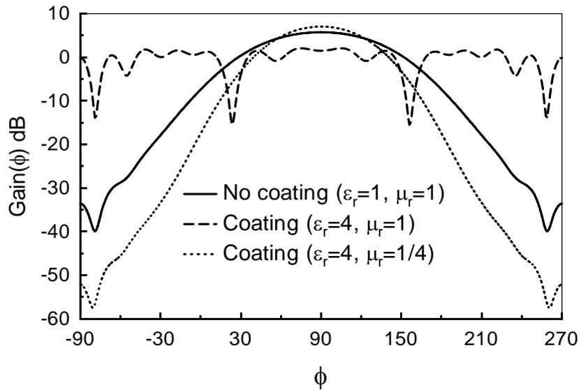
Figure 3: Radiation pattern for an axially slotted elliptic cylinder coated with different types of dielectric materials and coating thickness  $t = 0.25\lambda$ .
