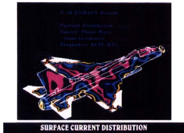
Figure 7. F16 surface currents from the GEMACS code.
