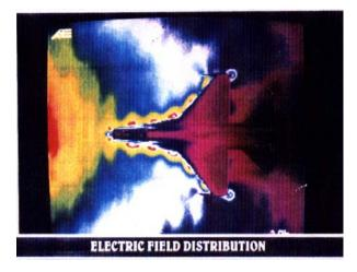
Figure 6. Test results for scale model F16. IR thermogram for normal incidence in the plane of the wings.
