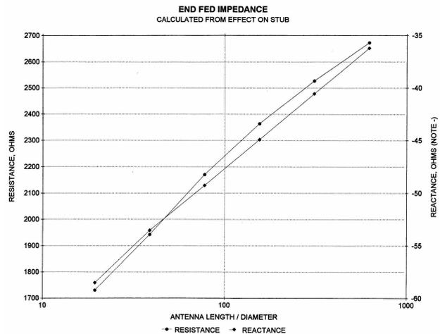
Fig. 6. Calculated end-feed impedance of a half-wave antenna used in the J-pole configuration. See text.
