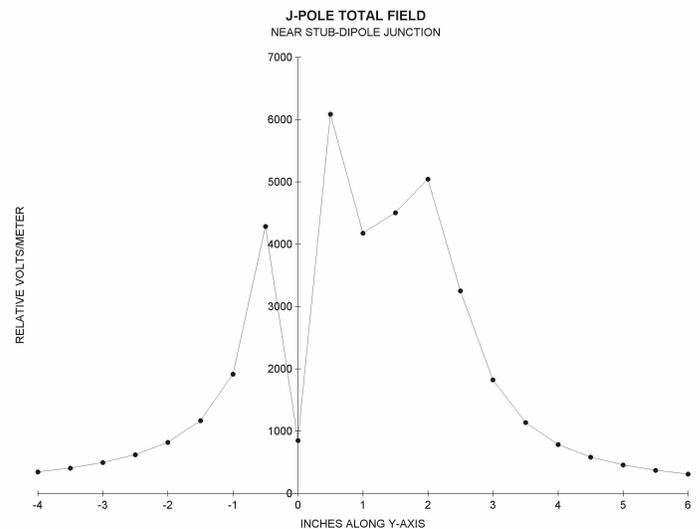
Fig. 4. E-field component of the near field close to the antenna and at the level of the antenna-U junction. The plane of the U is on the Y-axis. Maximum intensity is between the U arms, close to the side connected to the antenna. At approximately twice the U spacing from the arms, the field is nearly symmetrical.
