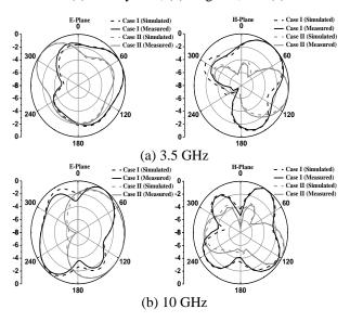
Fig. 8. Normalized radiation plots: (a) 3.5 GHz and (b) 10 GHz.
