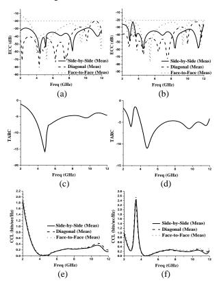
Fig. 10. MIMO/Diversity performance parameters: (a) ECC for Case I, (b) ECC for Case II, (c) TARC for Case I, (d) TARC for Case II, (e) CCL for Case I, and (f) CCL for Case II.
