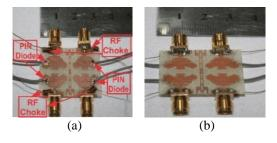
Fig. 3. Fabricated design: (a) front view and (b) back view.
