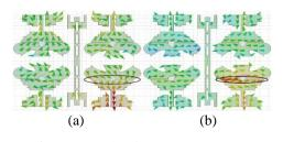
Fig. 4. Surface current density *J*-surf at 3.5 GHz: (a) Case I and (b) Case II.
