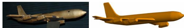
Fig. 1. Boeing 707 scale model in the compact range and laser scanned 3D CAD model in FEKO.
