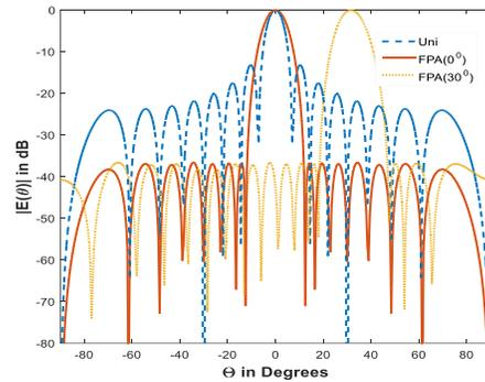
Fig. 3. SLL suppression in unscanned and scanned patterns.
