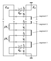
Fig. 4. Equivalent circuit of the half-loop segmented antenna.
