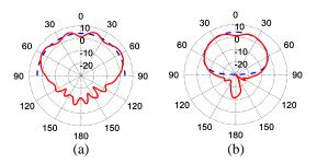
Fig. 8. Measured (solid) and simulated (dashed) radiation patterns of the antenna at 1.2276 GHz in: (a) xz or  $\varphi = 0^{\circ}$  and (b) yz or  $\varphi = 90^{\circ}$  planes.
