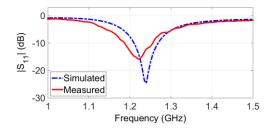
Fig. 9. Reflection coefficient magnitude of the antenna.
