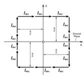
Fig. 5. The positions and orientations of the current moments on the segmented half-loop antenna.
