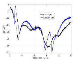
Fig. 5. Measured  $S_{11}$  in two states: 1-Diodes ON, 2-Diodes OFF.
