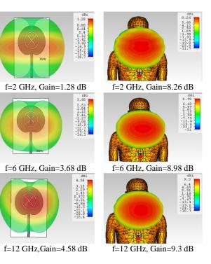
Fig. 6. Comparision of the antenna radiation patterns at different frequencies with human body and without human body.
