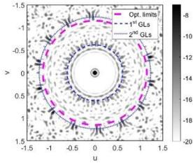
Fig. 7. Array factor of the array obtained from the 2<sup>nd</sup> optimization at 2 GHz. In thick dashed pink we have the limits of the sidelobe search for the optimization cost function. In thin dashed blue and dotted blue, we have the 1<sup>st</sup> and 2<sup>nd</sup> grating lobe regions, respectively.
