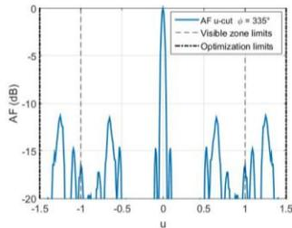
Fig. 4. Array factor representative u-cut ( $\phi = 335^\circ$ ) for the concentric ring array optimized at the  $\theta_s < 30^\circ$  zone, at 2 GHz (1<sup>st</sup> optimization).
