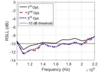
Fig. 5. RSLL in function of frequency of the 1<sup>st</sup> (continuous black), 2<sup>nd</sup> (dashed red) and 3<sup>rd</sup> (dotted blue) optimized array using the method described in Section IV.
