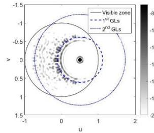
Fig. 6. Electric field of the array obtained from the 1<sup>st</sup> optimization with a steering of  $[\theta_s, \phi_s] = [30^\circ, 0^\circ]$ , calculated using the method from section IV, in the u-v space. In continuous black we have the visible zone. In dashed blue and dotted blue, we have the 1<sup>st</sup> and 2<sup>nd</sup> grating lobe regions, respectively.
