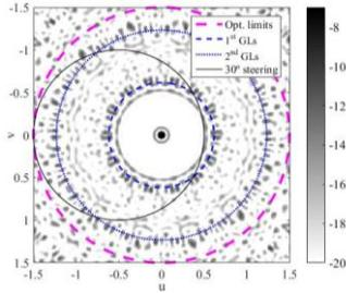
Fig. 3. Array factor of the array obtained from the 1<sup>st</sup> optimization at 2 GHz. In thick dashed pink we have the limits of the sidelobe search for the optimization cost function. In thin dashed blue and dotted blue, we have the 1<sup>st</sup> and 2<sup>nd</sup> grating lobe regions, respectively. In black we have the visible zone once steered to  $[\theta_s, \phi_s] = [30^\circ, 0^\circ]$ .
