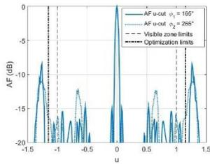
Fig. 8. Array factor representative u-cuts ( $\phi_1 = 165^\circ$  and  $\phi_2 = 265^\circ$ ) for the concentric ring array optimized at the  $(u d_{elem}/\lambda)^2 + (v d_{elem}/\lambda)^2 \leq 1.866^2$  zone, at 2 GHz (2<sup>nd</sup> optimization).
