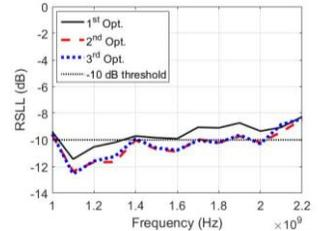
Fig. 5. RSLL in function of frequency of the 1<sup>st</sup> (continuous black), 2<sup>nd</sup> (dashed red) and 3<sup>rd</sup> (dotted blue) optimized array using the method described in Section IV.
