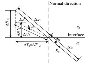
Fig. 3. The conformal process for Faraday loop path.
