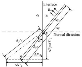
Fig. 5. The conformal process for Ampere loop path.
