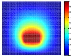
Fig. 8. The potential distribution without using conformal technique.
