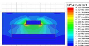
Fig. 11. The potential distribution of Fig. 10 model.
