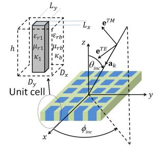
Fig. 1. A two-dimensional chiral grating slab excited by an obliquely incident TE and TM plane waves.
