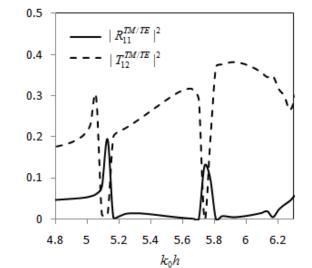
(b) TM reflection and transmission coefficients due to TE incident wave.
