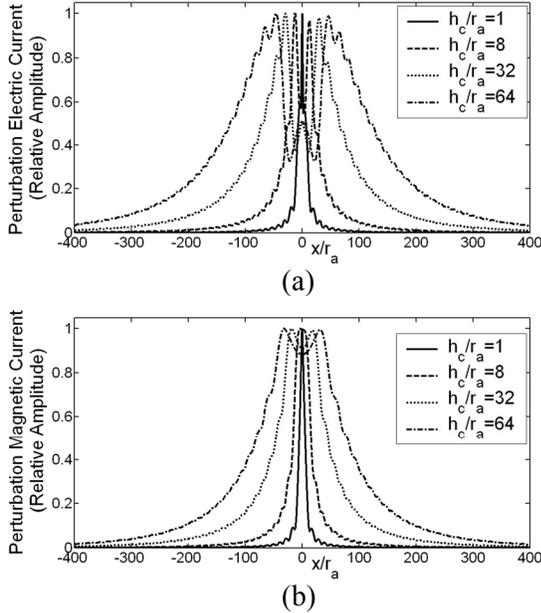
Fig. 8. Perturbation (a) electric and (b) magnetic currents on the flat surface for  $f=1$  GHz,  $\phi_i = 20^\circ$ ,  $r_a = 0.01$  m,  $x_c/r_a = 0.0$ ,  $\epsilon_1 = 15\epsilon_0$  F/m,  $\mu_1 = \mu_0$  H/m, and  $\sigma_1 = 0.01$  Sm $^{-1}$ .
