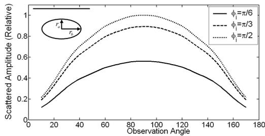
Fig. 12. Relative scattered amplitude from a cylindrical scatterer with elliptical cross-section for  $r_a = 0.02$  m,  $r_b = 0.01$  m,  $h_c / r_b = 1.0$ ,  $x_c / r_a = 0.0$ ,  $\epsilon_1 = 15 \epsilon_0$  F/m,  $\mu_1 = \mu_0$  H/m, and  $\sigma_1 = 0.01$  Sm $^{-1}$ .
