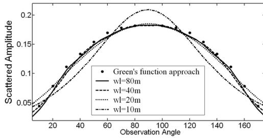
Fig. 11. Scattered amplitude from a cylindrical scatterer with circular cross-section for  $r_a = 0.3$  m,  $h_c = 1.7$  m,  $x_c / r_a = 0.0$ ,  $\epsilon_1 = 15 \epsilon_0$  F/m,  $\mu_1 = \mu_0$  H/m,  $\phi_i = 60^\circ$ ,  $f = 30$  MHz, and  $\sigma_1 = 0.01$  Sm $^{-1}$ .
