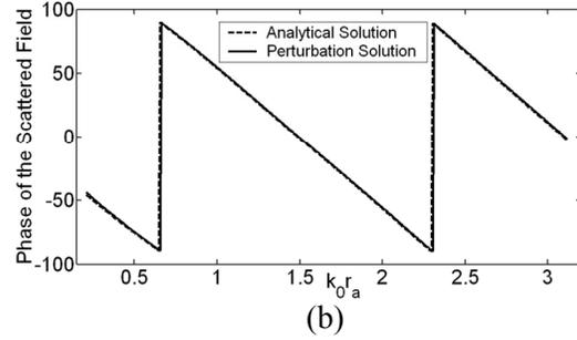
Fig. 9. Scattered field (a) normalized amplitude and (b) phase for  $r_a = 0.01$  m,  $\phi_i = 90^\circ$ ,  $h_c/r_a = 1.0$ ,  $x_c/r_a = 0.0$ ,  $wl/r_a = 500$ ,  $\epsilon_1 = \epsilon_0$  F/m, and  $\mu_1 = \mu_0$  H/m.
