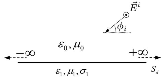
Fig. 2. The flat surface as a scatterer.
