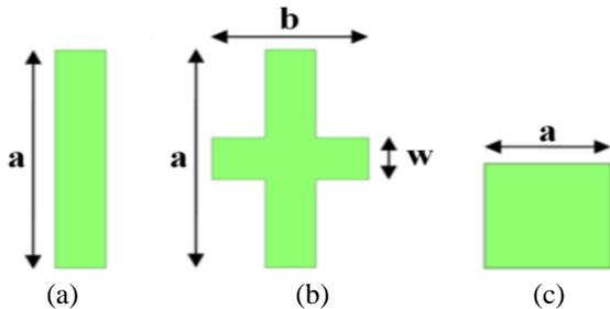
Fig. 12. Geometry of the investigated unit cells: (a) dipole, (b) cross, and (c) square.
