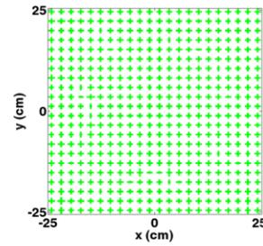
Fig. 20. MRA layout for  $D = 49$  cm and cross elements.
