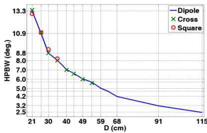
Fig. 17. Half-power beam-width vs.  $D$ .
