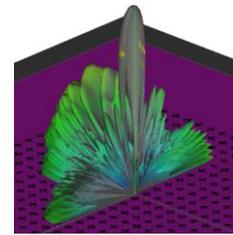
Fig. 21. Radiation pattern for  $D = 49$  cm in dB.
