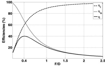
Fig. 5. E-plane efficiencies of the first feed.
