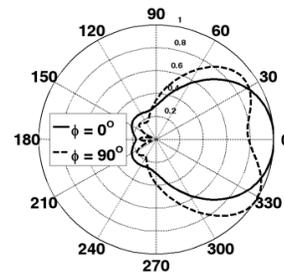
Fig. 3. Radiation patterns of the first feed.
