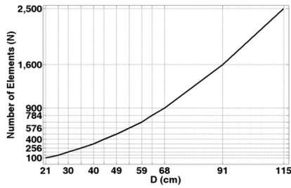
Fig. 14. Number of elements vs. reflector diameter.
