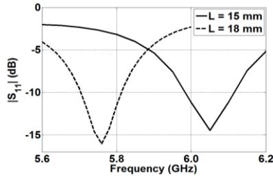
Fig. 8. Simulated  $|S_{11}|$  for the second feed.
