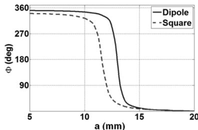
Fig. 13. Delay characteristics of unit cells.
