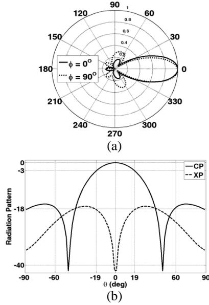
Fig. 10. Radiation pattern of the second feed: (a) Co-pol at orthogonal planes, and (b) Co- and X-pol at E-plane.
