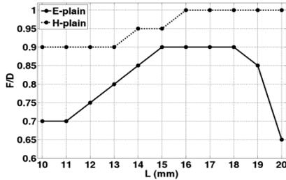
Fig. 7. F/D vs. L for the second feed.
