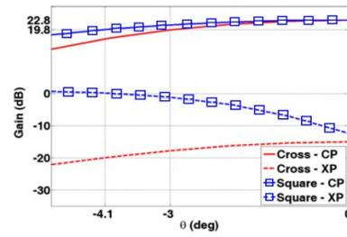
Fig. 19. Co-pol (CP) and X-pol (XP) gain patterns.
