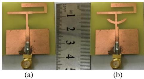
Fig. 2. Fabricated design: (a) Ant-1 and (b) Ant-2.
