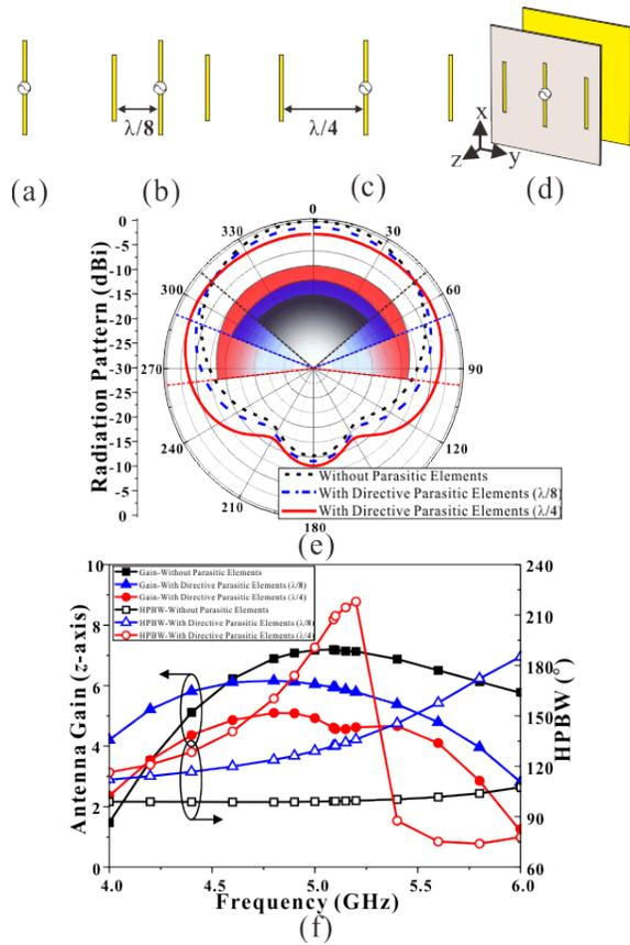
Fig. 2. Performance analysis of the antenna with or without parasitic elements: (a) a dipole antenna without parasitic element, (b) a dipole antenna with two parasitic elements of  $\lambda_0/8$ , (c) a dipole antenna with two parasitic elements of  $\lambda_0/4$ , (d) a simulation model for the proposed antenna, (e) radiation patterns and HPBWs with regard to the antenna structure, and (f) antenna gain at the main-beam direction and HPBW with regard to frequency variations.
