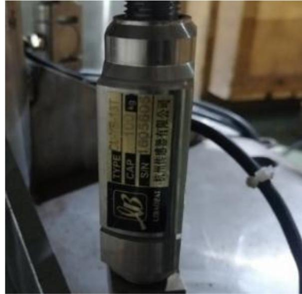
Fig. 2. CL-YB-13T/100kg force measuring sensor.
