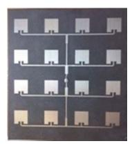
Fig. 14. Fabricated microstrip array antenna.
