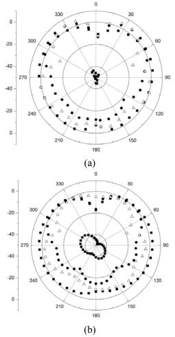
Fig. 5. Measured E-plane copolarization patterns (solid square: 2600MHz(both co- and X- pol); solid circle: 5800MHz; open uptriangle: 9300MHz). (a) Conventional monopole antenna, (b) proposed antenna.
