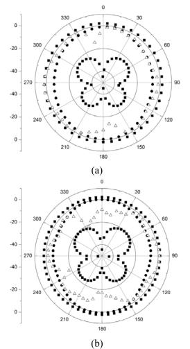
Fig. 6. Measured H-plane copolarization patterns (solid square: 2600MHz(both co- and X- pol); solid circle: 5800MHz; open uptriangle: 9300MHz). (a) Conventional monopole antenna, (b) proposed antenna.
