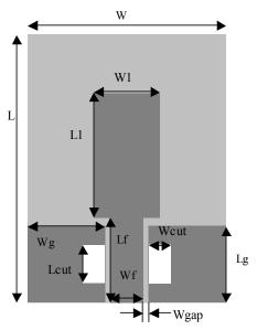
Fig. 1. The proposed monopole antenna.
