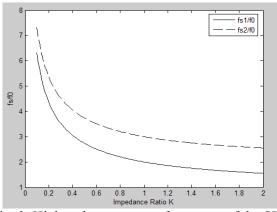
Fig. 3. High-order resonance frequency of the SIR.
