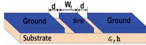
Fig. 2. Coplanar waveguide structure (CPW).
