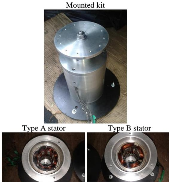
Fig. 7. Top view of prototypes A, in the left and B in the right; notice the 8 “poles” in Type A, and only 4 “poles” in Type B. A mounted kit is shown in the center, with a vertical rotor inserted in one of the casings.
