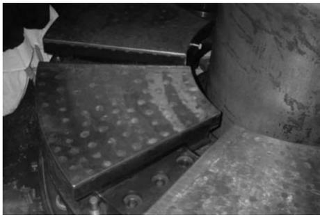
Fig. 3. Tilting-pads thrust bearing [8].
