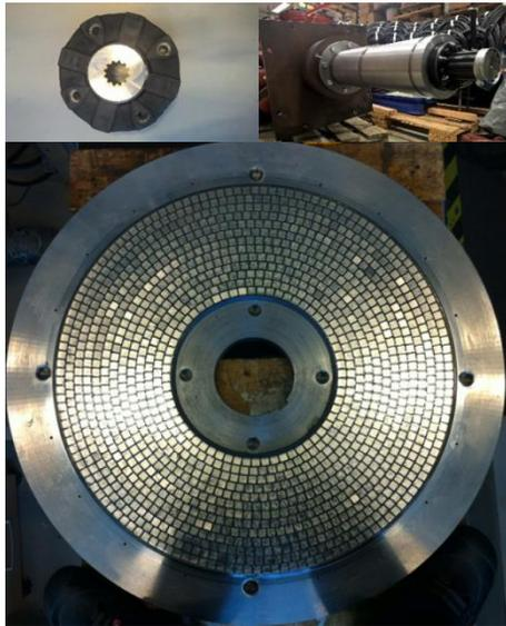
Fig. 2. (Top) Flexible coupling and driving end of the shaft. (Bottom) Permanent magnet thrust bearing rotor prior assembly. The details of the segmentation of the magnetic material can be appreciated.
