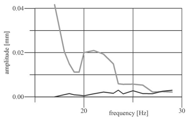
Fig. 6. The peak in the oscillation spectrum caused by the frequency of first flexural eigenmode as a function of rotation frequency.
