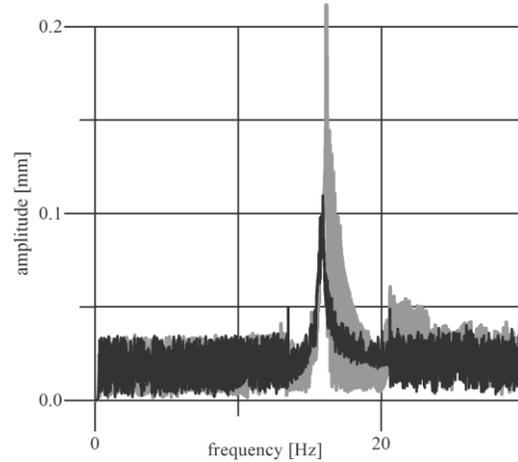
Fig. 1. Rotor displacement as a function of rotation frequency.
