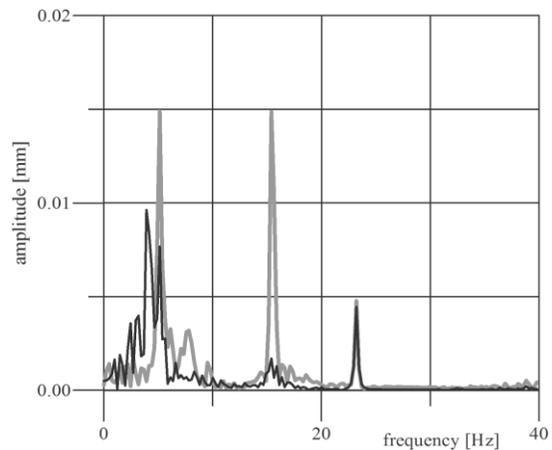
Fig. 5. Rotor oscillation spectrum at the rotation frequency of 23 Hz.
