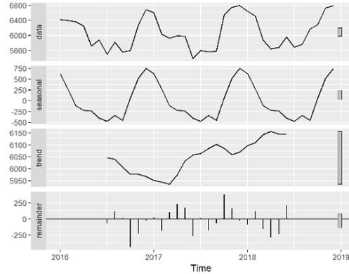
Fig. 2. The EMF data series (top) and its three additive components.
