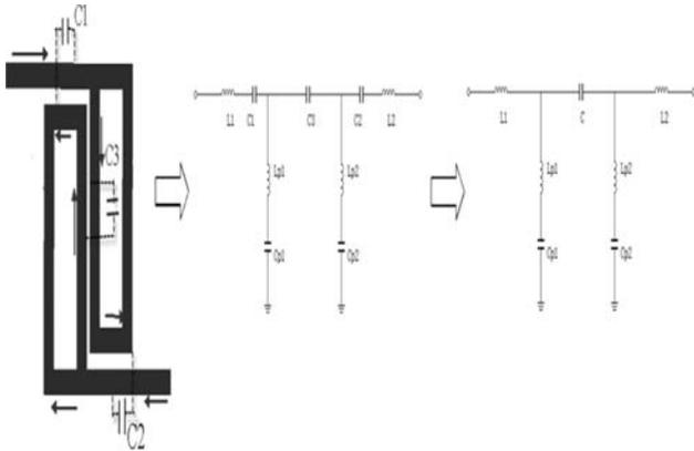
Fig. 4. The equivalent circuit of the unit cell.
