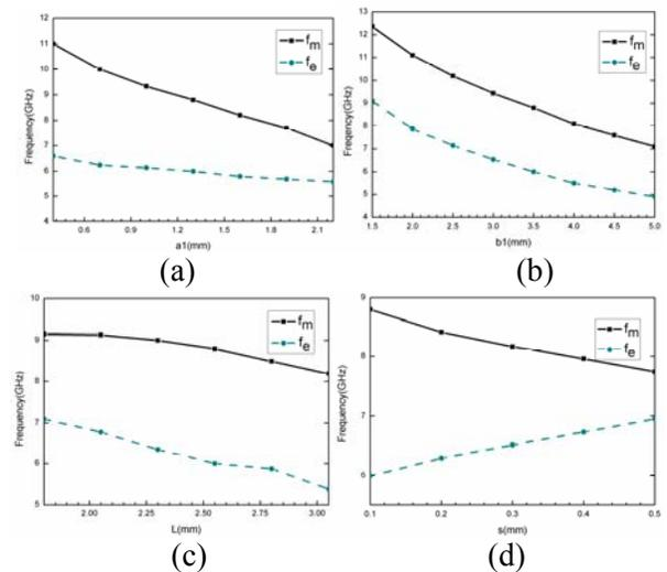
Fig. 6. Magnetic resonance frequency  $f_m$  and electric resonance  $f_e$  versus (a) the width of the ring, (b) the height of the ring, (c) the length of the branch, (d) the distance of the two P-like rings.
