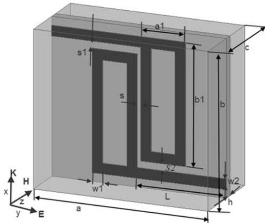
Fig. 1. Geometry of the double-P unit cell.
