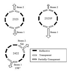
Fig. 25. Configuration methods of dual-beam modes.
