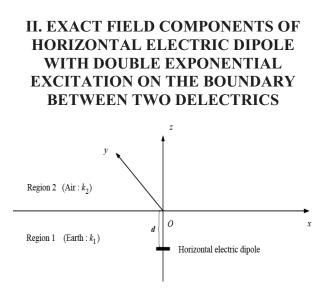
Fig. 1. Geometry of a horizontal electric dipole on the boundary between two dielectrics.
