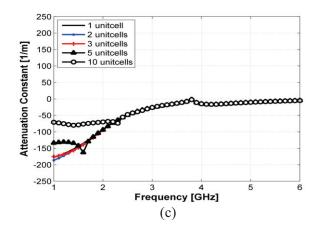
Fig. 6. (a) Schematic layout of a balanced and symmetric active CLRH-TL unit-cell design; simulated (b) phase constants  $\beta$  and (c) attenuation constants  $\alpha$  of 1, 2, 3, 5 and 10 unit cells of the balanced active CLRH-TL (figure adapted from [47]).
