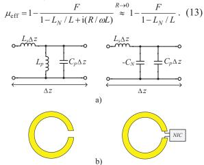
Fig. 10. (a) (left) An equivalent circuit model of a unit cell of a conventional epsilon-near-zero metamaterial transmission line, and (right) a broadband epsilon-near-zero metamaterial transmission line by replacing the periodic loaded inductance with a parallel negative capacitance [60]; (b) (left) a prototype of a SRR metamaterial with negative permeability, and (right) a scheme of a broadband SRR by embedding a negative impedance circuit at the gap.
