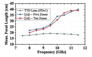
Fig. 6. Measured focal length of the lens discussed in Section III vs. frequency. For comparison the measured focal lengths of two non-TTD lenses reported in [14] are also presented.
