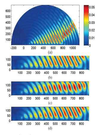
Fig. 3. |Re(E)| for the 20×20 Vivaldi antenna array in the *xz*-plane at 3.0 GHz with steering angle set at  $(\theta_s, \phi_s) = (60^\circ, 0^\circ)$ . (a) Computed using the conventional ABC with a hemispherical truncation surface, (b) same as (a) but plotted in a limited region for the purpose of comparison, (c) computed using the conventional ABC with a rectangular truncation surface, and (d) computed using the oblique ABC with a rectangular truncation surface.
