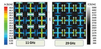
Fig. 13. Surface current and electric field distribution on the plane of the Jerusalem cross array at the two reflection resonances.
