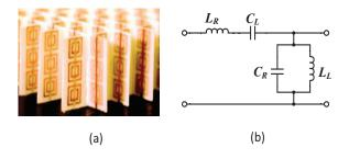
Fig. 1. Two most commonly studied metamaterial examples: (a) a wire (provides  $-\varepsilon$ ) and SRR (provides  $-\mu$ ) array (figure adapted from [3]), and (b) a unit cell of composite Left-Hand/Right-Hand Transmission Line (CLRH-TL).
