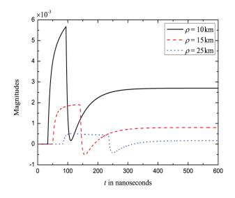
Fig. 3. Exact electric field  $E_{2\phi}(\rho,t)$  on the boundary in air of a horizontal electric dipole with the relative permittivity of the earth  $\varepsilon = 8$ .
