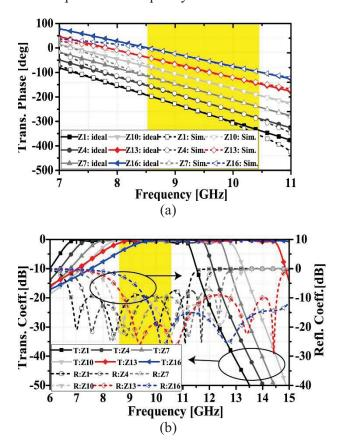
Fig. 4. (a) The simulated phase responses of the time delay units occupying the different zones of the MEFSS-based microwave lens discussed in Section III and (b) the magnitudes of the transmission and reflection coefficients of the different pixels of the lens.
