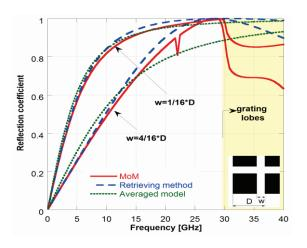
Fig. 7. Reflection coefficients obtained with different models. Parameters: D=10 mm and different w.
