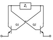
Fig. 9. A schematic of a negative impedance circuit example based on Linvill's configuration. The output impedance approximates to be  $Z_{in}$ =- $Z_L$ .
