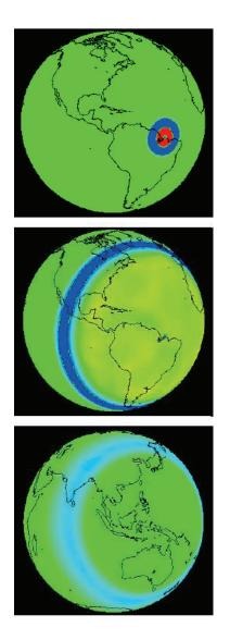
Fig. 1. Snapshot visualizations of round-the-world EM propagation below 1 kHz as calculated by a 3-D FDTD model, including details of the Earth's topography, oceans, and isotropic ionosphere (figure courtesy of [7]).
