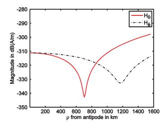
Fig. 5. Magnitudes of the components  $H_{\theta}$  and  $H_{\phi}$  at f=100 Hz with a=6378 km,  $\phi = \pi/4$ ,  $\sigma_g = 10^{-5}$  S/m, h=85 km, and  $\beta = 0.3$  km<sup>-1</sup>.
