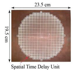
Fig. 5. Photograph of the fabricated prototype of an MEFSS-based planar microwave lens using band-pass MEFSSs (after [15]).
