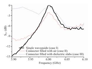
Fig. 5. The experimental results of the transmission parameters  $(S_{21})$ .
