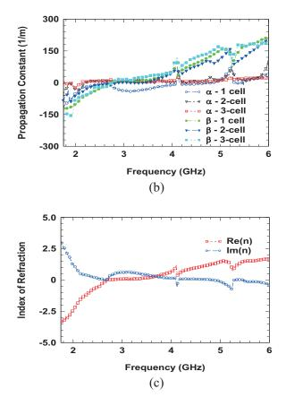
Fig. 4. (a) Simulated and (b) measured propagation constants of the active CLRH-TL incorporating tunneling diodes with one, two and three unit cells; (c) extracted refractive index from the measured one unit cell results with a time dependence convention  $e^{j\omega t - \gamma z}$  (figure adapted from [46]).
