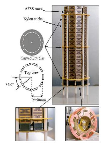
Fig. 20. Antenna structure and installation.
