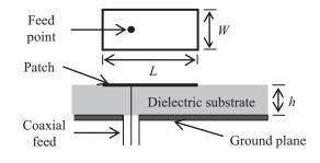
Fig. 1. Model of rectangular MSA.
