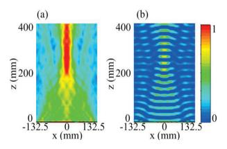
Fig. 18. (a) Simulation result of the distribution of the transmitted electric fields amplitude of pure cross-pol component for the converging lens, and (b) simulation result of the distribution of the transmitted  $E_y$  component.
