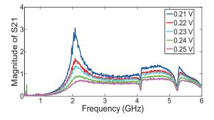
Fig. 5. Measured transmission  $S_{21}$  of the one-unit cell active CLRH-TL with the tunneling diode biased from 0.21 to 0.25 V. The level of loss compensation/gain can be controlled by the bias voltage.
