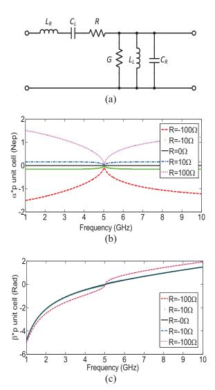
Fig. 2. (a) Equivalent circuit model of a unit cell of a CLRH-TL metamaterial, (b) calculated attenuation constant  $\alpha$  ( $\alpha$ >0-loss,  $\alpha$ =0-lossless,  $\alpha$ <0-gain), and (c) phase constant  $\beta$  ( $\beta$ >0-RH,  $\beta$ <0-LH) (figure adapted from [45]).
