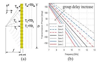
Fig. 2. (a) Side view of an MEFSS-based true-timedelay microwave lens and (b) the phase response of the different spatial time delay units occupying the aperture of the lens.
