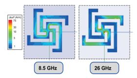
Fig. 15. Surface current on the plane of the spiral cross array at the two reflection resonances.
