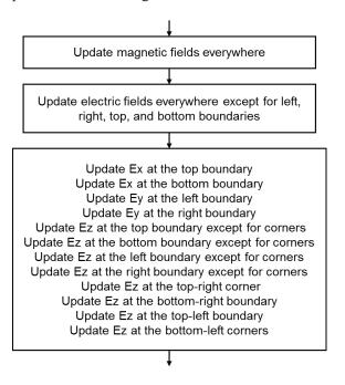
Fig. 3. Conventional field update process for treatment of periodic boundary conditions.
