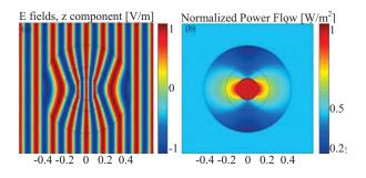
Fig. 2. (a) Electric field distributions of the cylindrical EM concentrator, and (b) normalized power flow distribution of the concentrator.
