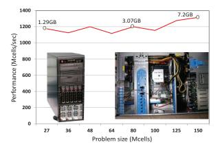
Fig. 7. Performance of the 5110P Phi coprocessor for the parallel FDTD code with the regular size of problems.
