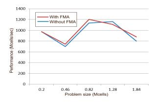
Fig. 8. Performance of the 5110P Phi coprocessor for the parallel FDTD code with the small size of problems.
