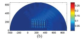
Fig. 6. |E| in the  $\phi = 0^{\circ}$  plane for H-pol excitation at 3.02 GHz and steering angle  $\theta_s = 60^{\circ}$  and  $\phi_s = 0^{\circ}$ . (a) The NRL array itself, and (b) the NRL array with a radome.
