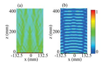
Fig. 19. (a) Simulation result of the distribution of the transmitted electric fields amplitude of pure cross-pol component for the diverging lens, and (b) simulation result of the distribution of the transmitted  $E_v$  component.
