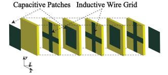
Fig. 3. Topology of a unit cell of a band-pass MEFSS of the type reported in [12]. This MEFSS has a fourth-order bandpass response and is composed of 7 metal layers and six dielectric layers.
