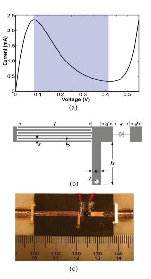
Fig. 3. (a) Current voltage relation (I-V curve) of the Germanium tunneling diode. The differential negative resistance appears at 0.15-0.3 V. (b) Schematic of a designed active CLRH-TL unit cell in microstrip configuration incorporating the resonant tunneling diode. The dimensions are: a=2.5 mm, d=1.5 mm, l=9.7 mm, w=1 mm, s=0.2mm,  $l_s=5.9$  mm, r=0.3 mm. (c) Photo of a fabricated single unit cell of the active CLRH-TL (figure adapted from [46]).
