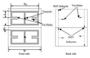
Fig. 23. Layout of the unit cell.
