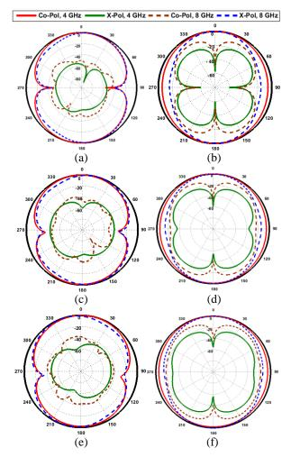
Fig. 6. Co-polar and cross-polar normalized radiation patterns at 4 GHz and 8 GHz for: (a) *E*-plane at  $0^{\circ}$ , (b) *H*-plane at  $0^{\circ}$ , (c) *E*-plane at  $45^{\circ}$ , (d) *H*-plane at  $45^{\circ}$ , (e) *E*-plane at 90°, and (f) *H*-plane at 90°.
