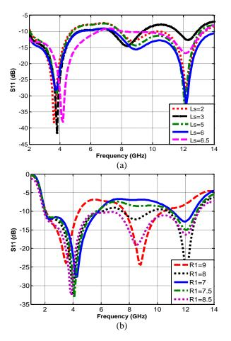
Fig. 4. Reflection coefficient of the antenna for: (a) different values of  $L_s$ , and (b) different values of  $R_1$ .
