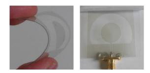
Fig. 3. Schematic of the fabricated antenna.
