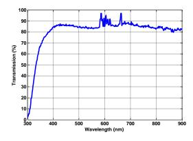
Fig. 2. Measured optical transparency of the antenna for various wavelengths.
