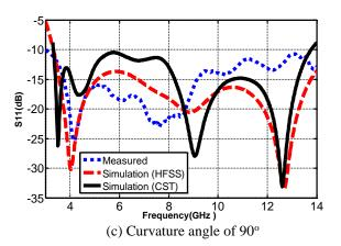
Fig. 5. Reflection coefficient of the antenna for several curvature angles.
