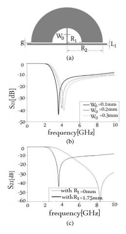
Fig. 1. (a) Schematic diagram of the designed filter, (b) simulation results for  $S_{21}$  with variation of  $W_0$ , and (c) simulation results for  $S_{21}$  with variation of  $R_1$ .
