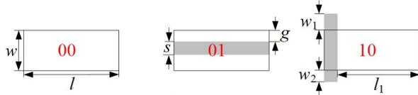
Fig. 1. Elements proposed for the 2-bit FTS scheme.
