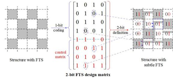
Fig. 2. Structure coding for the 2-bit FTS scheme.
