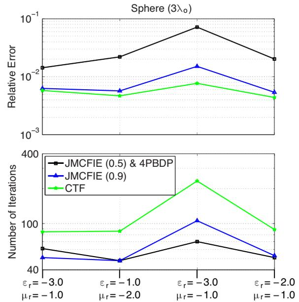
Fig. 3. The relative error and the number of BiCGStab iterations (for  $10^{-3}$  residual error) required in numerical solutions of scattering problems involving a sphere of radius 0.3 m at 3 GHz.
