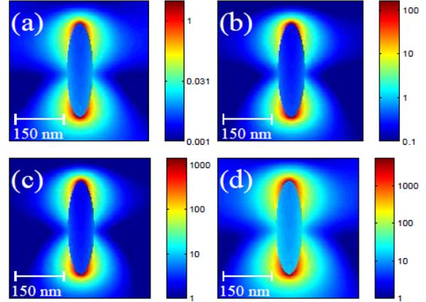
Fig. 8. Intensity distributions for a prolate spheroid. The distributions are given for various half-beam angles: (a)  $\alpha = 15^\circ$ , (b)  $\alpha = 30^\circ$ , (c)  $\alpha = 45^\circ$ , and (d)  $\alpha = 60^\circ$ .
