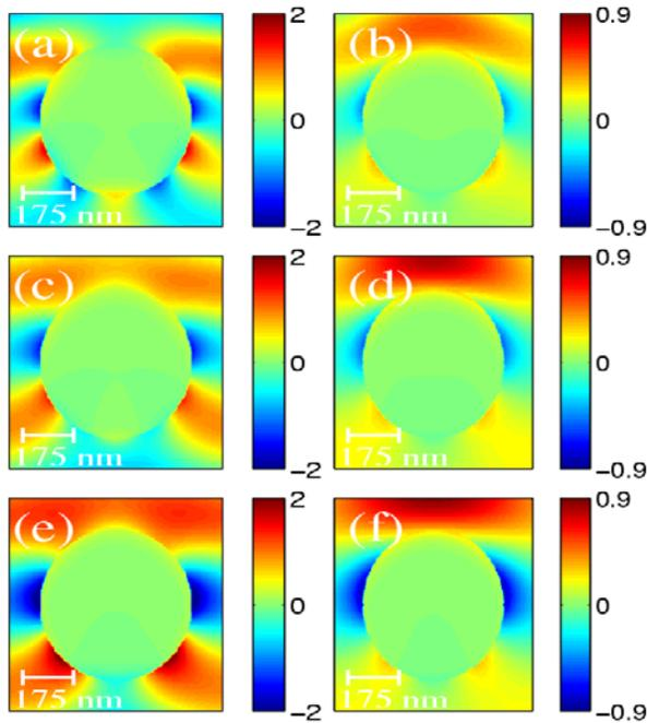
Fig. 3.  $E_x(x, 0, z)$  on the  $x$ - $z$  plane for various  $[\alpha(^{\circ}), \lambda(\text{nm})]$ : (a)  $E_x(x, 0, z)$  for  $[5, 400]$ , (b)  $E_x(x, 0, z)$  for  $[60, 400]$ , (c)  $E_x(x, 0, z)$  for  $[5, 500]$ , (d)  $E_x(x, 0, z)$  for  $[60, 500]$ , (e)  $E_x(x, 0, z)$  for  $[5, 600]$ , and (f)  $E_x(x, 0, z)$  for  $[60, 600]$ .
