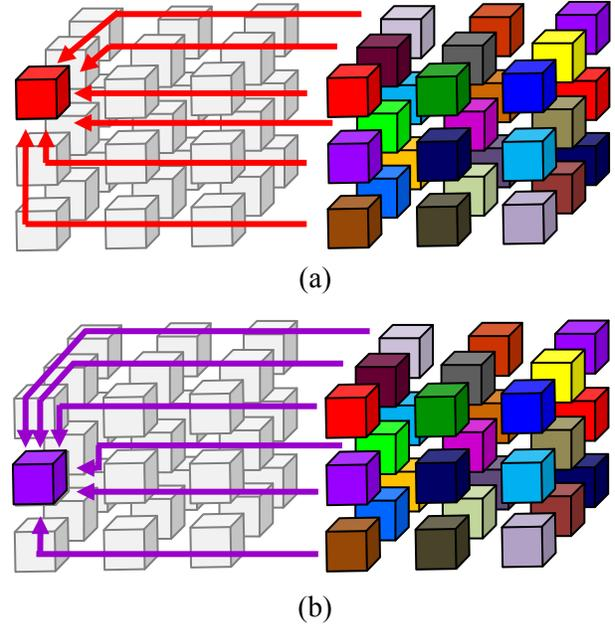
Fig. 4. Pictorial description of the parallelization of the computation of  $\mathbf{F}(\mathbf{r}_i, t_n)$ , at time step  $t_n$  in scheme 2. (a)  $\mathbf{F}(\mathbf{r}_i, t_n)$  for all  $\mathbf{r}_i$  that reside in the red box (on the left) is computed in parallel. (b)  $\mathbf{F}(\mathbf{r}_i, t_n)$  for all  $\mathbf{r}_i$  that reside in the purple box is computed in parallel.
