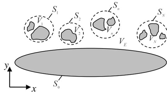
Fig. 1. Reference geometry for the discussion of the concept of stochastic macro-modeling.
