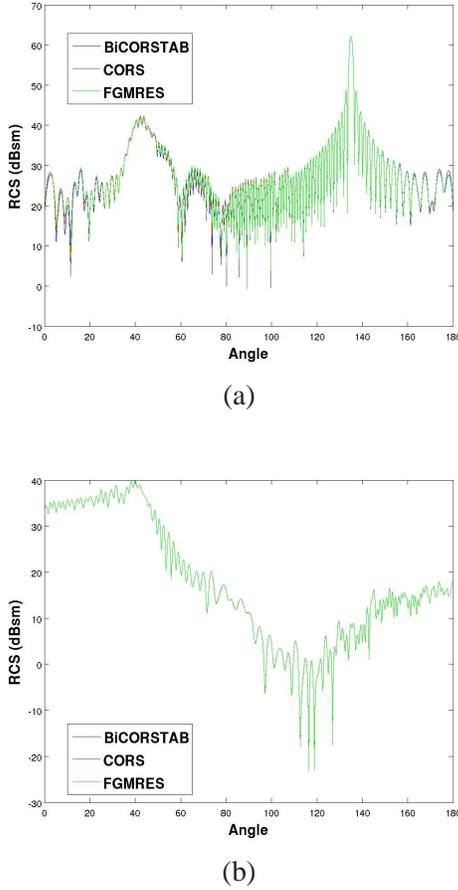
Fig. 3. Comparative curves of the radar-cross-section (RCS) calculation for (a) the cavity problem, and (b) the paraboloid problem.
