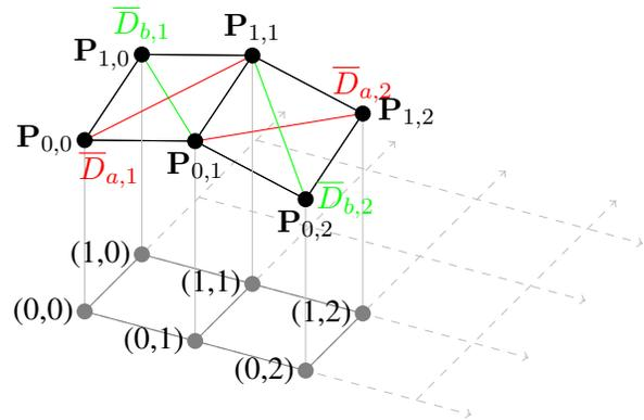
Fig. 2. Triangle construction from elevation map point set. Points  $P$  illustrate the heights at a given matrix coordinate. The diagonals  $\bar{D}$  illustrate possible diagonals for the triangular tessellation. Four possible selection strategies can be applied: left-upper-right-lower (red), left-lower-right-upper (green), or choosing the diagonal by length (shorter or longer).
