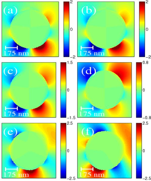
Fig. 7.  $E_z(x, 0, z)$  on the  $x$ - $z$  plane: (a) plane wave at  $0^\circ$ , (b) focused beam with  $\alpha = 0^\circ$ , (c) focused beam with  $\alpha = 45^\circ$ , (d) focused beam with  $\alpha = 60^\circ$ , (e) plane wave at  $30^\circ$ , and (f) plane wave at  $60^\circ$ .
