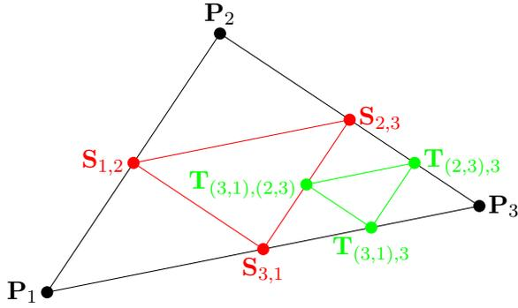
Fig. 1. Sierpinski tessellation of a triangle. Points  $S$  are the edge bisection points of the original triangle. Points  $T$ , also edge bisection points, illustrate one further step in the refinement process.
