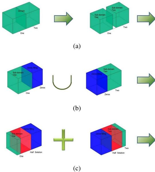
Fig. 6. Parallel FDTD computation with update after  $N$  time steps. (a) Two adjacent sub-domains, analyzed in parallel, (b) Zero padded extensions (blue boxes) of each sub-domain. The extensions protrude into the adjacent sub-domain, (c) Superposition of the overlapping solutions over each sub-domain, that includes the green and red boxes.
