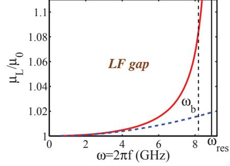
Fig. 3. Permeability  $\hat{\mu}_L/\mu_0$  in the LF gap. Solid (red) and dashed (blue) lines correspond, respectively, to the exact [Eq. (4)], and approximate [Eq. (44)] expressions of  $\hat{\mu}_L(\omega)/\mu_0$ ; a relative error of less than 5% is achieved for  $\omega_b \equiv 2\pi \times 1.28 \text{ GHz} < \omega < \omega_{\text{res}} = 2\pi \times 1.45 \text{ GHz}$ .
