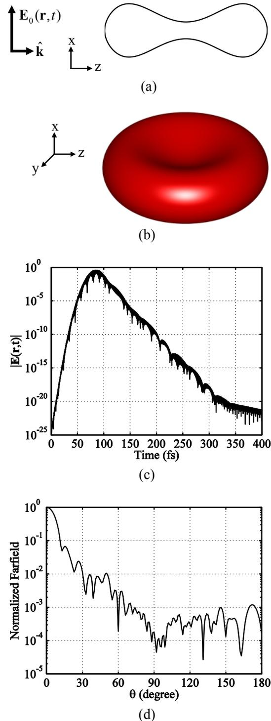
Fig. 7. Analysis of light scattering from an RBC. (a) Cross-section of the RBC model along the  $xz$ -plane and the plane wave excitation. (b) Three dimension view of the model. (c) The amplitude of the transient electric field induced at the center of the RBC. (d) Normalized amplitude of the electric far-field on the  $xz$ -plane.
