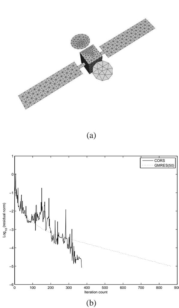
Fig. 1. Example 3: a satellite. (a) The discretized mesh. (b) The convergence history of the CORS vs. the restarted GMRES methods.
