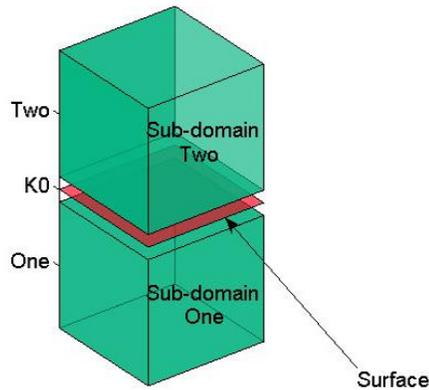
Fig. 3. Diakoptics-on-the-fly: two sub-domains with a planar seam.
