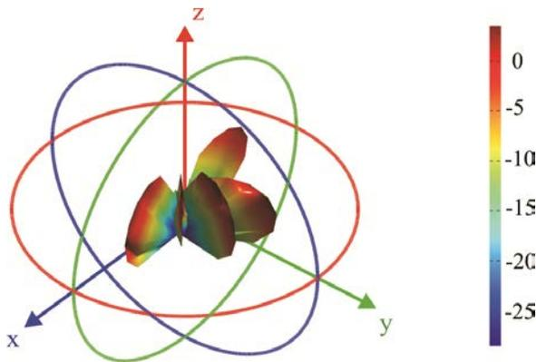
Fig. 23. Radiation pattern at final iteration (irregular distribution): AWGN model with SNR 70dB.
