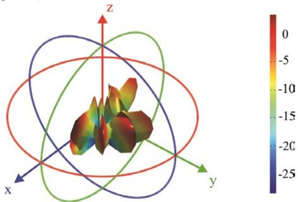
Fig. 13. Radiation pattern at final iteration (irregular distrib.): UWN model with SNR 30dB.
