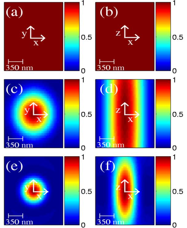
Fig. 2. (a)  $E_x(x, 0, z)$  on the  $x$ - $y$  plane for  $\alpha = 0^\circ$ , (b)  $E_x(x, 0, z)$  on the  $x$ - $z$  plane for  $\alpha = 0^\circ$ , (c)  $E_x(x, 0, z)$  on the  $x$ - $y$  plane for  $\alpha = 30^\circ$ , (d)  $E_x(x, 0, z)$  on the  $x$ - $z$  plane for  $\alpha = 30^\circ$ , (e)  $E_x(x, 0, z)$  on the  $x$ - $y$  plane for  $\alpha = 60^\circ$ , and (f)  $E_x(x, 0, z)$  on the  $x$ - $z$  plane for  $\alpha = 60^\circ$ .
