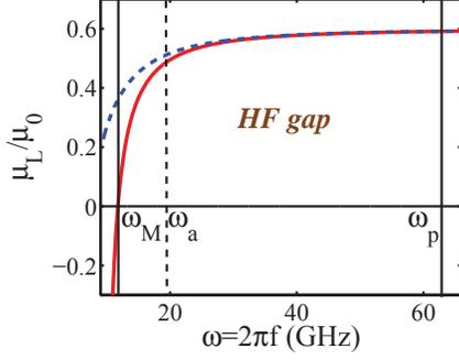
Fig. 2. Permeability  $\hat{\mu}_L/\mu_0$  in the HF gap. Solid (red) and dashed (blue) lines correspond, respectively, to the exact [Eq. (4)] and approximate [Eq. (39)] expressions of  $\hat{\mu}_L(\omega)/\mu_0$  in this band. The approximation produces a relative error less than 5% for  $\omega_a \equiv 2\pi \times 3.1 \text{ GHz} < \omega < \omega_p = 2\pi \times 10 \text{ GHz}$ .
