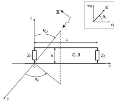
Fig. 1. Transmission line struck by a plane wave.
