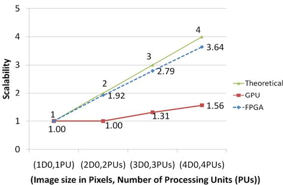
Fig. 9. Scalability of algorithm on FPGA vs. GPU.
