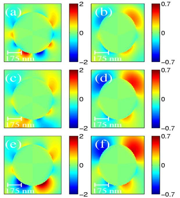
Fig. 4.  $E_z(x, 0, z)$  on the  $x$ - $z$  plane for various  $[\alpha(^{\circ}), \lambda(\text{nm})]$ : (a)  $E_z(x, 0, z)$  for  $[5, 400]$ , (b)  $E_z(x, 0, z)$  for  $[60, 400]$ , (c)  $E_z(x, 0, z)$  for  $[5, 500]$ , (d)  $E_z(x, 0, z)$  for  $[60, 500]$ , (e)  $E_z(x, 0, z)$  for  $[5, 600]$ , and (f)  $E_z(x, 0, z)$  for  $[60, 600]$ .
