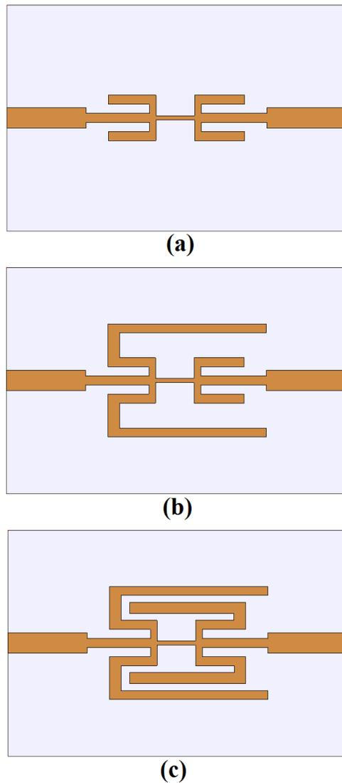
Fig. 2. (a) Microstrip filter with a pair of C-shaped strips, (b) the filter with left-side W-shaped and C-shaped strips, and (c) the proposed filter structure.
