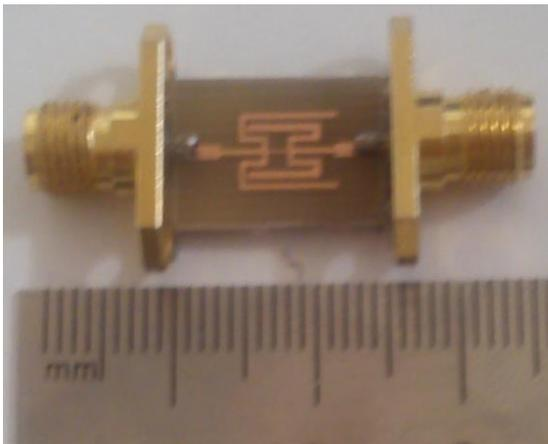
Fig. 6. Photograph of the fabricated microstrip filter.
