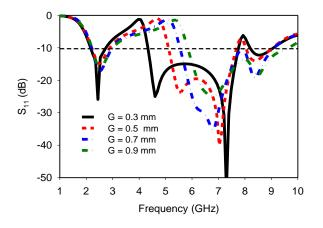
Fig. 6. Simulated return loss characteristics of configuration C for various width C.
