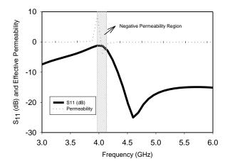
Fig. 7. Comparison of extracted real parts of effective permeability and  $S_{11}$  (dB).
