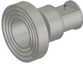
Fig. 1. Model of WR430 CATR feed.
