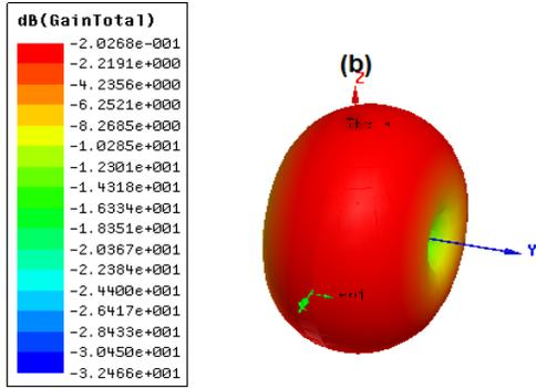
Fig. 4. 3D radiation patterns of two antenna elements.
