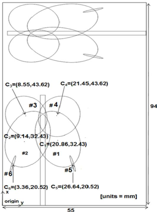
Fig. 2. The top view of the proposed antenna.
