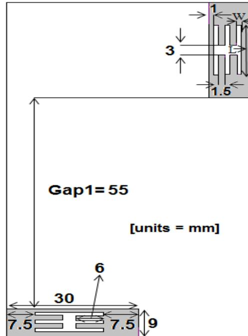
Fig. 3. The bottom view of the proposed antenna.
