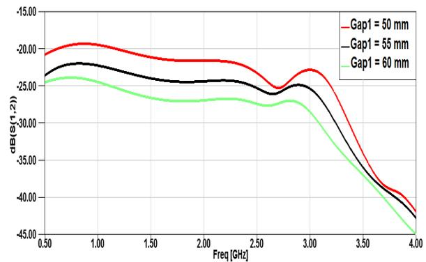
Fig. 13. Simulated S(1,2) with different value of Gap1.
